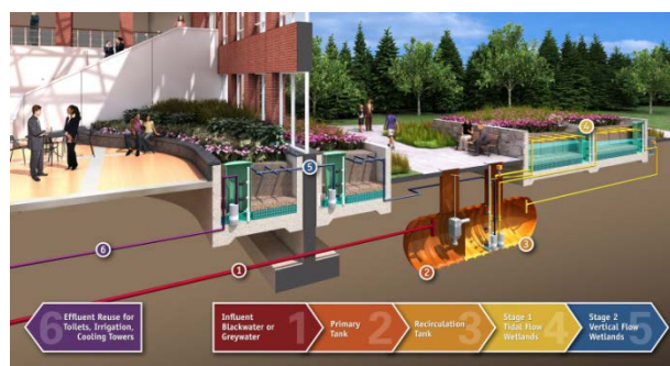
Figure 4. Worrell’s Living Machine—Constructed Wetlands in An Upscale Office Building
